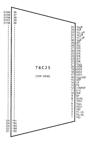
\*: The above diagram shows the pin configuration of the LSI Chip, not that of the tape carrier package.
