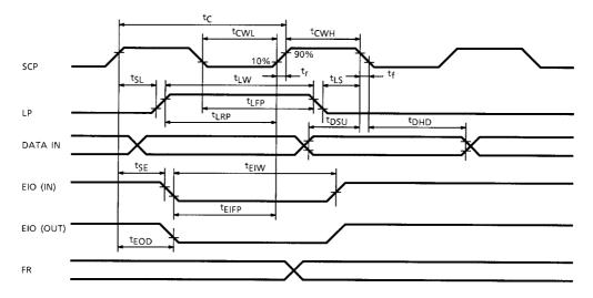
TEST CONDITIONS (1) ( $V_{SS} = 0 \text{ V}, V_{DD} = 4.5 \text{ to } 5.5 \text{ V}, V_{CC} = 14 \text{ to } 42 \text{ V}, Ta = -20 \text{ to } 75^{\circ}\text{C}$ )
